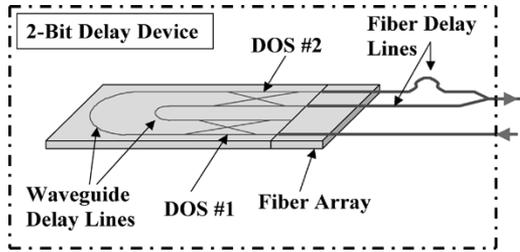
Fig. 1. Schematic of the 2-bit reconfigurable delay device.
