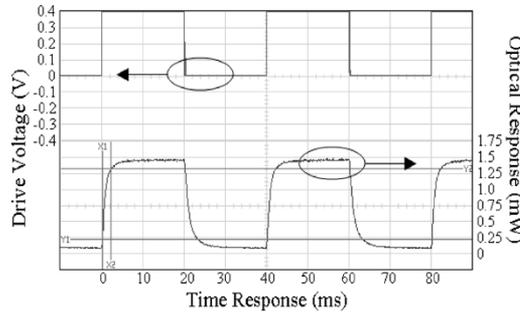
Fig. 2. Switching speed measurement results of the  $2 \times 2$  DOS switch.
