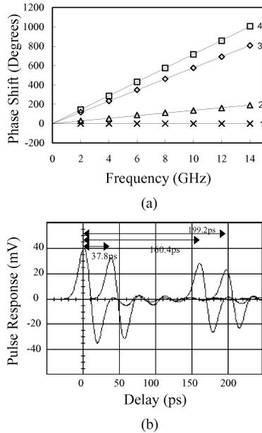
Fig. 4. (a) Phase versus RF frequency measurement results for each of the four delay states. (b) Time response of a femtosecond laser pulse through the device.
