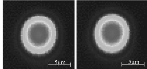
Fig. 3. Near-field images of TE (left) and TM (right) polarizations emanating from the 2-bit device.
