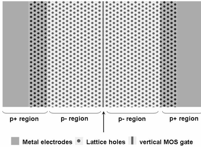
Fig. 1 Schematic top view of MOS-capacitor-based silicon photonic crystal waveguide
