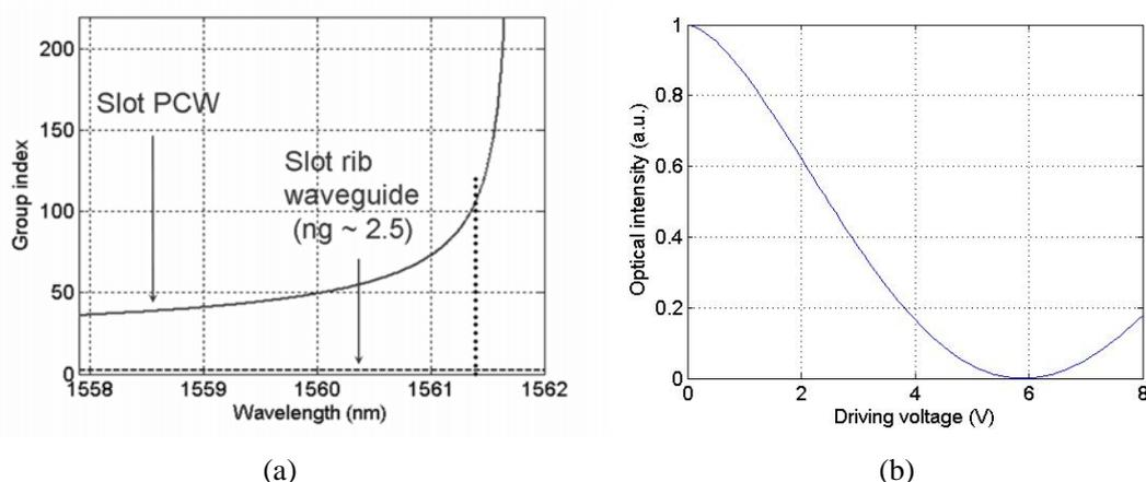
Fig. 3 (a) Group indices simulated at different wavelengths (b) DC modulation curve
