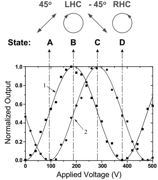
Fig. 4. Measured output of the 45°-tilted-polarization component versus the modulating voltage. • the principal axis of the quarter-wave plate is 45° tilted; ■ the principal axis of the quarter-wave plate is vertical; — the curve of the Sine function.
