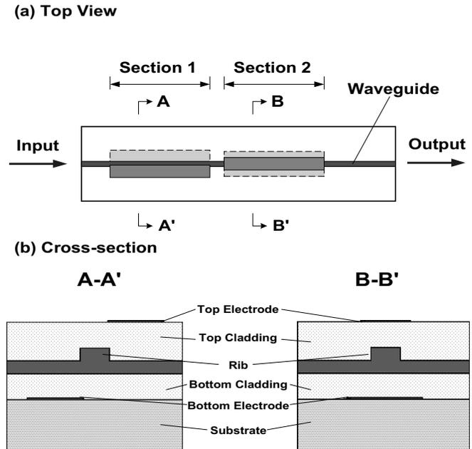
Fig. 1. Schematic diagram of the EO-polymer-based optical circular-polarization modulator.
