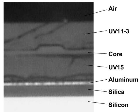
Fig. 2. Cross section of the polymeric waveguide.
