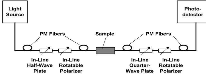
Fig. 3. Schematic diagram of the optical measuring setup.
