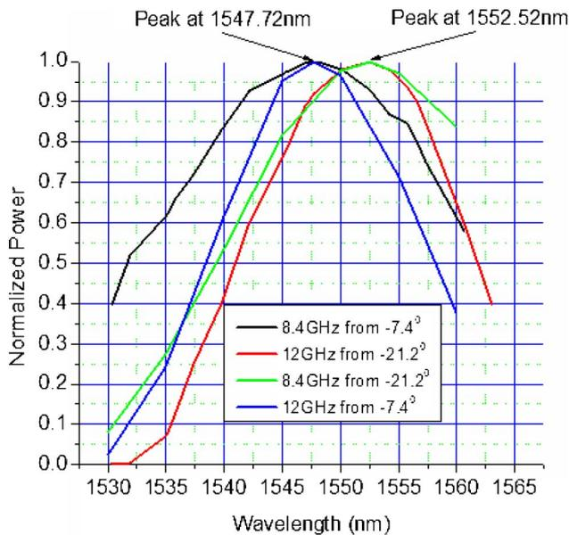
Fig. 4. (Color online) Signal power measured at the photodetector versus wavelength. The signal power peaks appear at 1547.72 nm for 8.4 and 12 GHz signals placed at  $-7.4^\circ$  and at 1552.52 nm for 8.4 and 12 GHz signals placed at  $-21.2^\circ$ .
