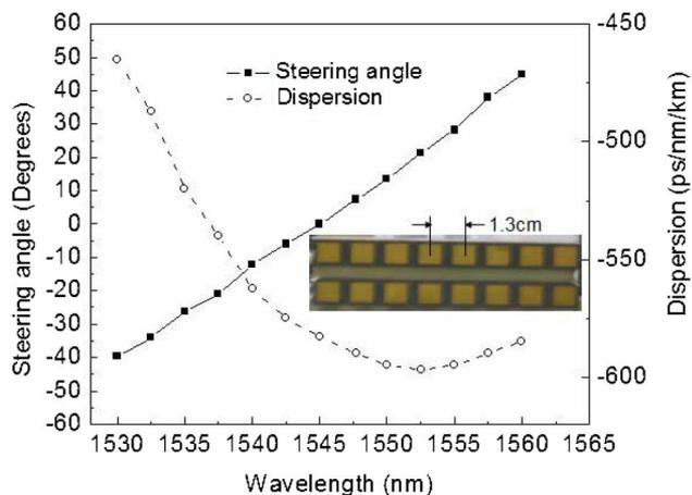
Fig. 2. (Color online) Solid curve shows the calculated steering angle of the beam as a function of wavelength. The dashed curve shows the measured dispersion coefficient of the PCF. The inset shows the X-band antenna array with an element spacing of 1.3 cm.
