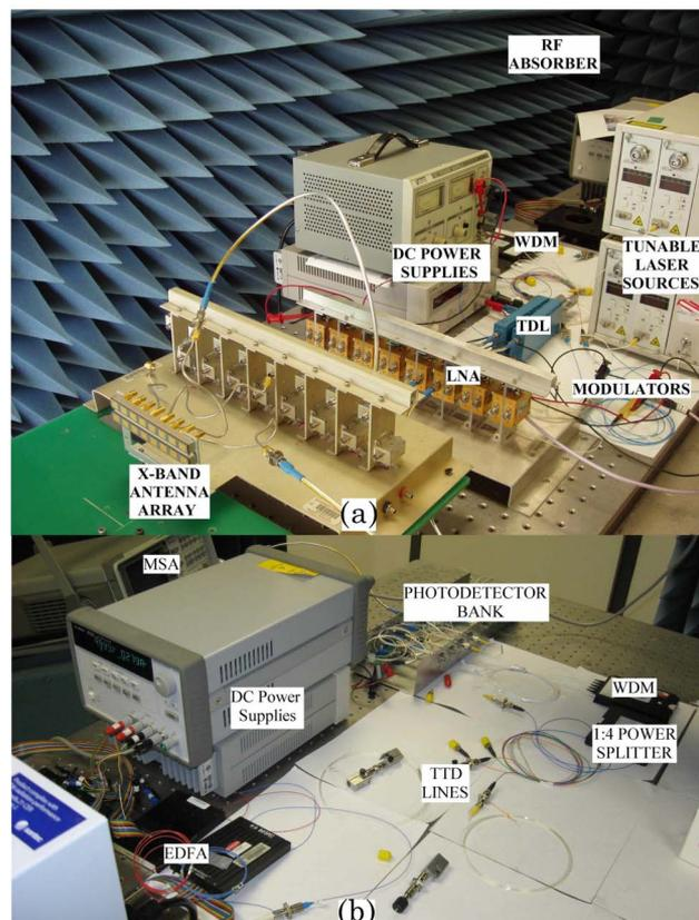
Fig. 3. (Color online) Schematic of the experimental setup. (a) Photograph showing the RF reception and electro-optical conversion section of the overall setup. (b) Photograph showing the TTD lines and signal processing section of the overall setup. The output from the modulators in (a) are connected to the inputs of EDFAs in (b). (The RF sources and the transmitting horn antennas of the setup are not shown.)
