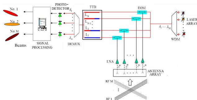
Fig. 1. (Color online) Structure of the receiving mode with multiple incoming beams. DEMUX, demultiplexer.
