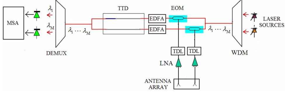
Fig. 1. Schematic of the experimental setup: LNA: low noise amplifier, WDM: wavelength division multiplexer, TDL: tunable delay line, MSA: microwave spectrum analyzer, WDM: wavelength division multiplexer, TTD: true-time-delay, EDFA: Erbium doped fiber amplifier (The RF sources and the transmitting horn antennas of the setup are not shown in the figure).
