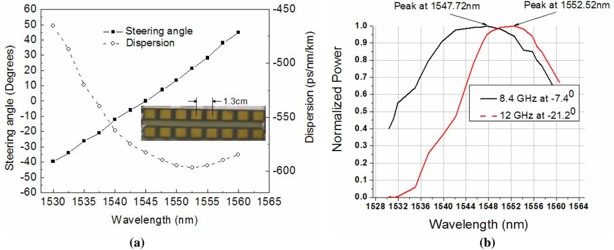
Fig. 2. (a) The solid curve shows the calculated steering angle of the beam as a function of wavelength. The dashed curve shows the measured dispersion coefficient of the PCF. The inset shows the X-band antenna array with an element spacing of 1.3cm. (b) Signal power measured at the photodetector vs. wavelength. The signal power peaks appear at 1547.72nm and 1552.52nm for 8.4GHz and 12GHz respectively.
