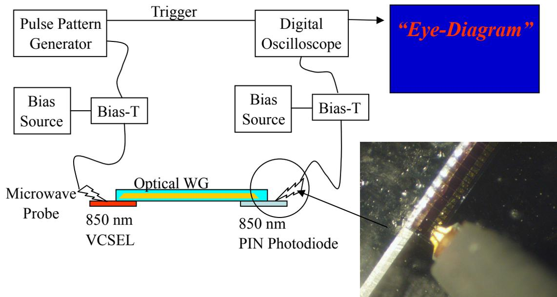
Fig.5 Schematic diagram of the measurement setup for the assembled optical system
