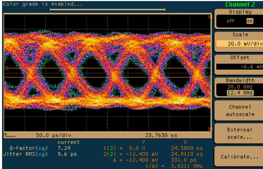
Fig.6 Measured 10Gbps eyediagram with a Q-factor of 7.24
