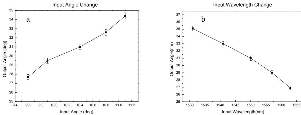
Fig.9. The beam steering experiment result based on the (a) input angle change and (b) input wavelength change.
