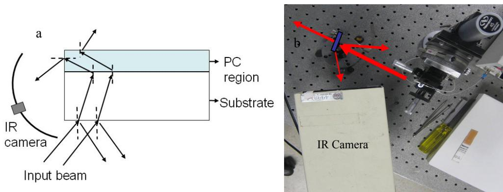
Fig.7 (a) Schematic view and (b) experimental setup of the beam steering test
