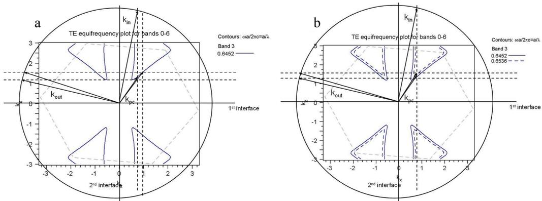
Fig.3 EFC analysis for (a) the input angle change and (b) input wavelength change
