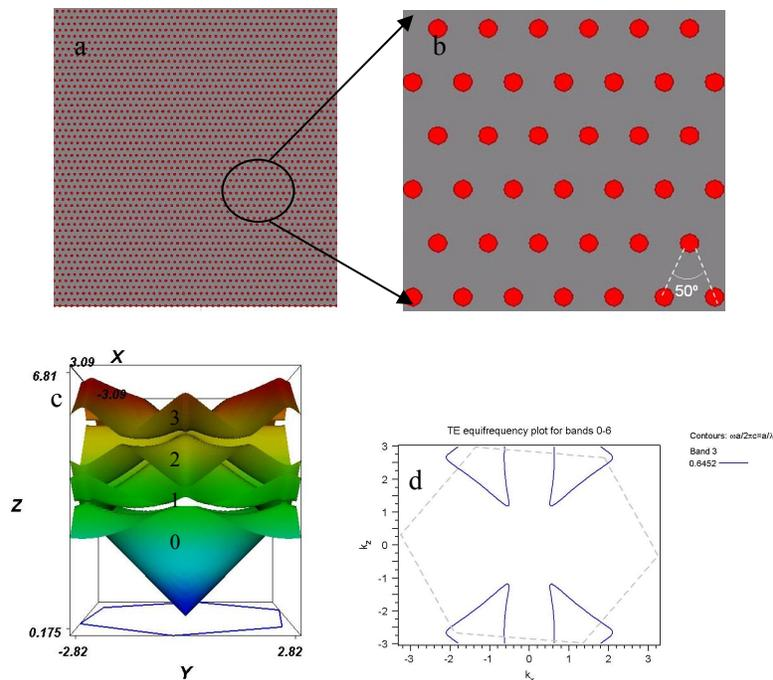
Fig.1. (a) (b) Layout of the photonic crystals in xoz plane. (c) 3D band structure of the polymer based photonic crystals. The x,y axis represents  $k_x$  and  $k_z$ , respectively. z represents the frequency. (d) The EFC (Equi-frequency Contour) at certain frequency( $\omega a/2\pi c=a/\lambda=0.6452$ ) for band 3.
