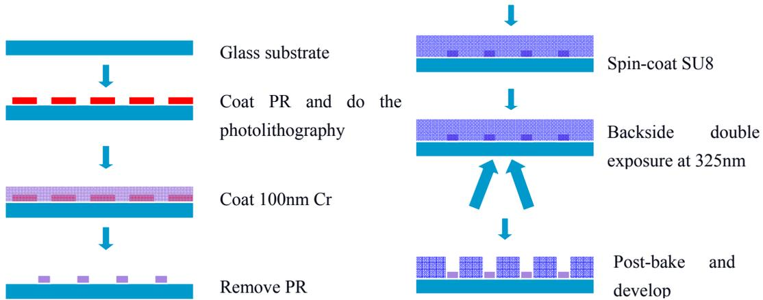
Fig.5 The scheme of fabrication of horizontally stacked photonic crystal on the glass substrate.
