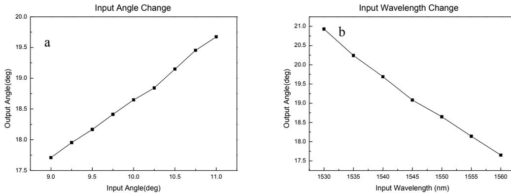
Fig.4 The output angle change vs (a) input angle change and (b) input wavelength change.
