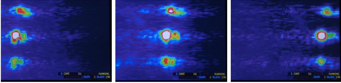
Fig.8 Typical IR camera view of the steering output beams for three different input angles at 1.55 $\mu$ m wavelength.
