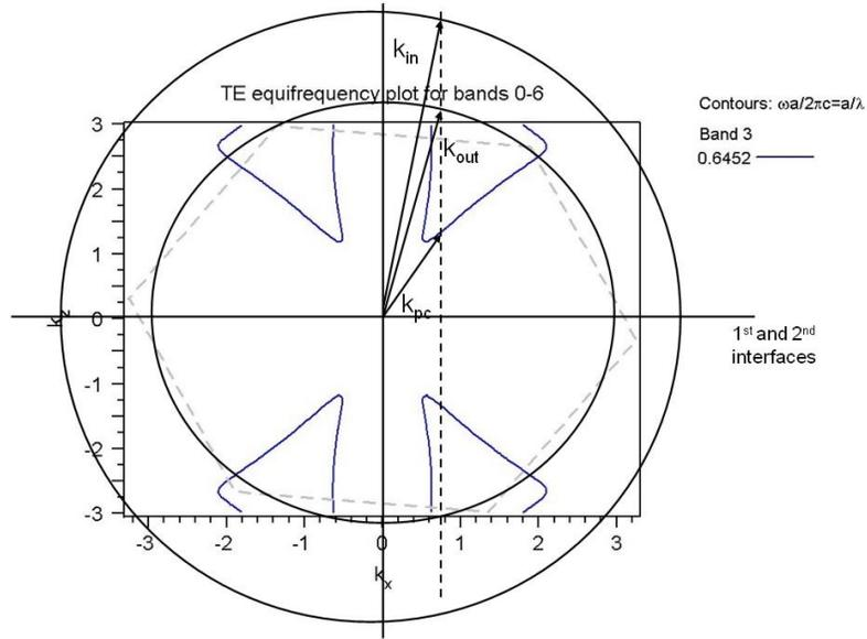
Fig. 2. Analysis of the refraction process when the input and output surfaces are parallel.
