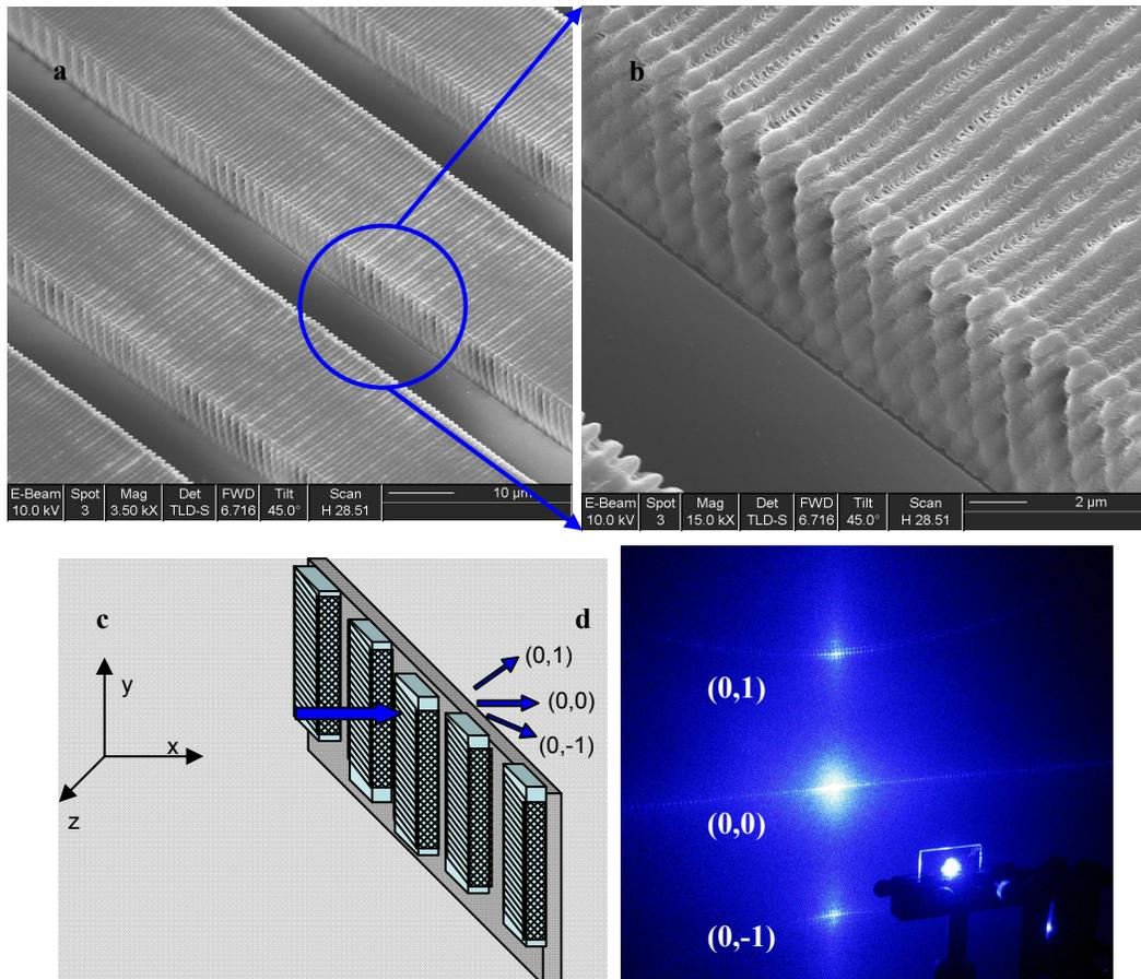
Fig. 6 (a) low and (b) high magnification view SEM pictures of the horizontally stacked photonic crystal structures fabricated using SU8. (c) The schematic laser diffraction setup. (d) The 442nm laser diffraction pattern of the fabricated photonic crystals.
