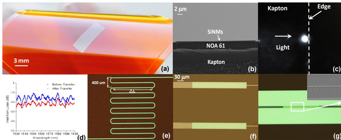
Fig. 2 (a) Transferred SiNM waveguide showing good flexibility. (b) SEM image of the cross section of the waveguide after transfer. (c) The output spot captured by a topside down IR camera. (d) The insertion loss of 7 mm SiNM based flexible waveguide (red) and the SOI based waveguide (blue) (e) The structure used to measure the propagation loss of the waveguide. (f) Transferred 1 by 6 MMI couplers. (g) Transferred Photonic crystal waveguide
