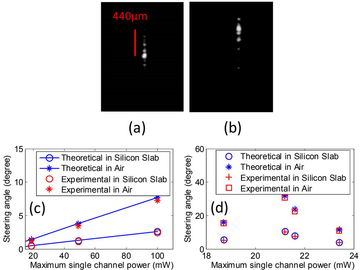
Fig. 4. Top down IR images of the far field viewed at the end of the silicon nanomembrane slab (a) non-steered beam, (b) beam steered at  $2.5^\circ$  in silicon. Steering angle vs maximum power applied in a single channel for both the silicon slab and in air (c) without reset and (d) with reset.
