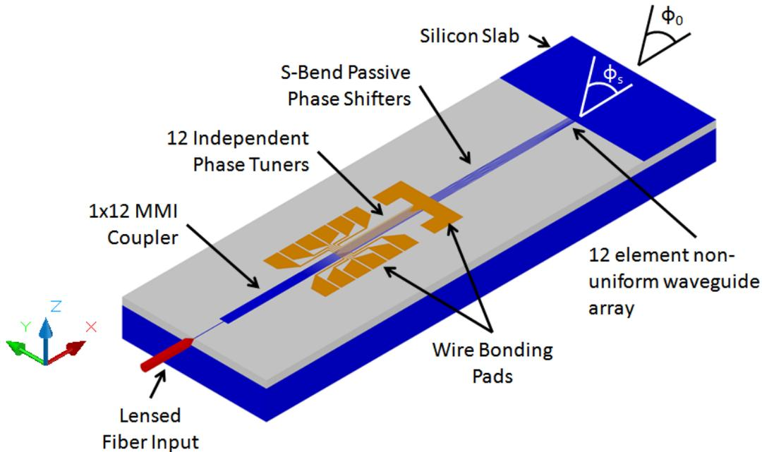
Fig. 2. A schematic of the silicon waveguide based optical phased array.
