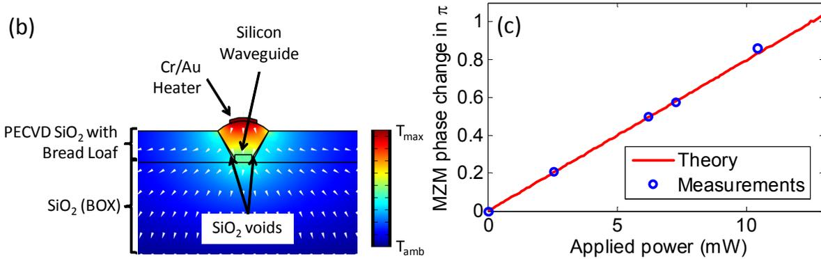
Fig. 3 (a) SEM cross section of a heater over its waveguide with oxide voids caused by PECVD bread-loading. (b) Simulated thermal profile using PECVD SiO<sub>2</sub> with bread loafing that shows reduction in lateral heat transfer and more efficient heating of silicon waveguide. (c) Electrical power vs phase change in MZM showing P<sub>π</sub> value of 12.4mW.
