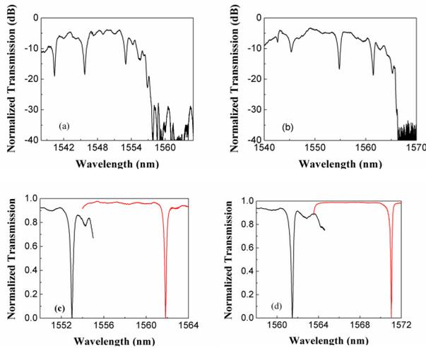
Figure 2. Experimental W1 PCW transmission spectrum in water with coupled (a) L13 and (b) L21 microcavities. Experimental spectra showing shift of resonance mode closest to the band edge in (a) and (b) in (c) and (d) respectively in water (black) versus glycerol (red).
