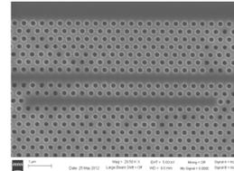
Figure 1. SEM of L21 PC microcavity side coupled to a W1 PCW.
