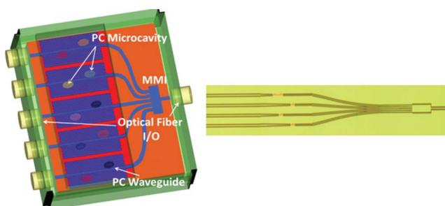
**Fig. 1** (a) Generalized schematic of the test system on chip with integrated  $1 \times x$ MMI and PC microcavities coupled to PC waveguides. On each of the  $x$  output arms of the MMI, multiple PC microcavities are arrayed. Each microcavity is coated with a different target receptor biomolecule, each responsive to its specific conjugate, as indicated by a different color. (b) Stitched microscope image of  $1 \times 4$ MMI device studied here.
