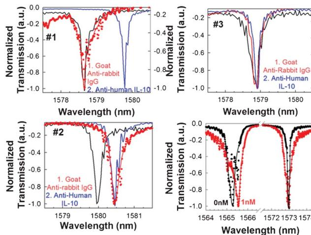
**Fig. 5** Resonance wavelength shift or none thereof observed in the (a)–(c) L13 PC microcavities in arms 1–3 of the  $1 \times 4$ MMI when probe antibodies goat anti-rabbit IgG in PBS and rat anti-human IL-10 in PBS are added in sequence and (d) arm 4 of the  $1 \times 4$ MMI with 1 nM of probe antibodies of goat anti-rabbit IgG in PBS.
