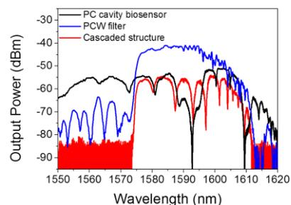
Fig. 4. Measured spectra for single PC cavity (black), single PCW filter (blue), and cascaded structure of these 2 devices (red).
