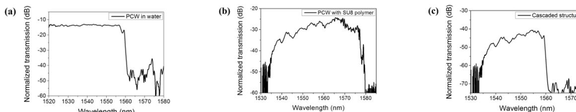
Fig. 2. Waveguide transmission spectra of (a) PCW in water (b) PCW with SU8 polymer, in water and (c) predicted series connected devices in (a) and (b).
