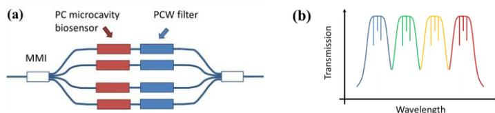
Fig. 3. (a) Schematic of multiplexed biosensor microarray with single output port. (b) Predicted transmission spectrum of the device in (a), with different colors corresponding to different PC microcavity biosensors.
