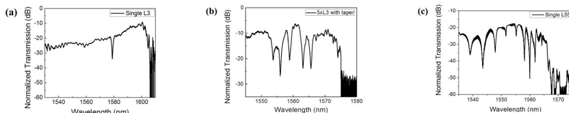
Fig. 1. Transmission spectrum in water for a W1 PCW coupled to (a) a single L3 PC microcavity, (b) series connected five L3 PC microcavities in cascaded PCWs and (c) a single L55 PC microcavity. Spectra are taken in water from biosensing perspective.
