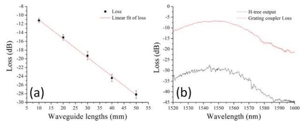
Figure 2. Optical measurements, (a) propagation loss of single-mode waveguide on adhesively bonded silicon nanomembrane determined by varying waveguide lengths using the cut-back method. (b) transmission spectra of the H-tree optical distribution (black) and the two grating couplers for input and output (red).
