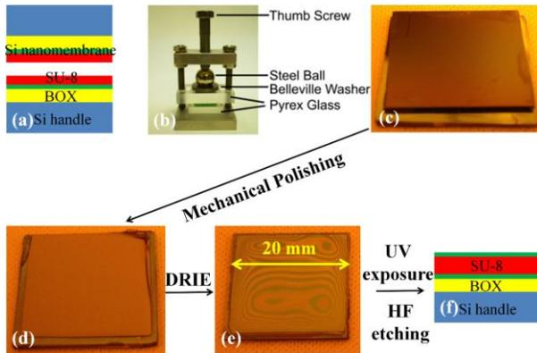
Figure 1. The process flow for bonding silicon nanomembrane onto another SOI chip, (a) schematic of the material stack structure, (b) the home-made bonder used for adhesive bonding, (c) the bonded two SOI chips, (d) polishing the silicon handle to  $\sim 100\mu\text{m}$ , (e) removing the remaining silicon handle with DRIE, (f) schematic of a silicon nanomembrane bonded to a SOI chip.
