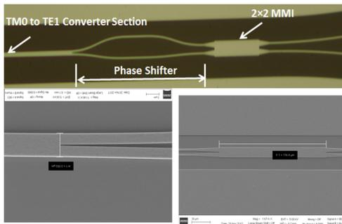
Fig. 5: (a) Microscope image of the polarization rotator. (b) the section where the TE1 mode splits into its two 180-degree shifted TE0 components (The SEM is flipped vertically to match with the microscope image in (a)). (c) Top view SEM images showing (a) the 2x2 multimode interference power splitter section
