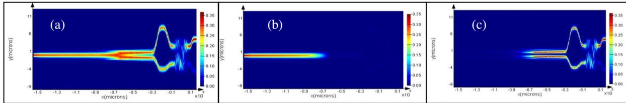
Fig. 2: (a) 3D FDTD simulation showing the electric field intensity magnitude across the complete device with TM0 input on the left side and TE0 output on the right side. (b) shows the electric field intensity magnitude of TM components of the propagating wave. As observed also from (c), complete conversion from TM to TE occurs near the center of the structure. First, TM0 to TE1 conversion after which it splits into two arms.
