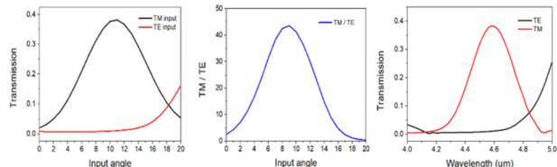
Fig. 4: 2D FDTD simulated transmission for a TM-polarization selective grating coupler versus (a) fiber incident angle and (b) incident wavelength in SoS operating around  $\lambda=4.55\mu\text{m}$
