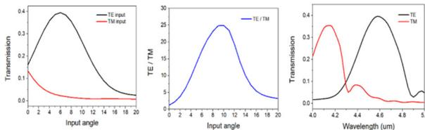
Fig. 3: 2D FDTD simulated transmission for a TE-polarization selective grating coupler versus (a) fiber incident angle and (b) incident wavelength in SoS operating around  $\lambda=4.55\mu\text{m}$
