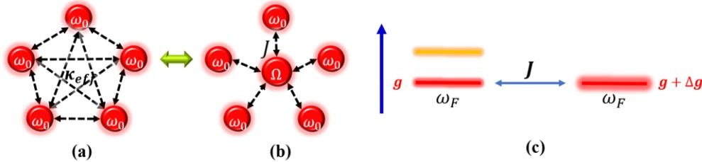
**Fig. 1.** Schematic representation of  $N$  coupled cavities that are mutually coupled to each other. System in (a) supports two super modes ( $\omega_0 - \kappa_{eff}$  and  $\omega_0 + (N-1)\kappa_{eff}$ ). One can achieve such a coupled system via adiabatic coupling to a central cavity  $\Omega$  and increasing its gain. (b) Schematic of  $Q$ -enhancing of the fundamental one through increasing the gain in central cavity.
