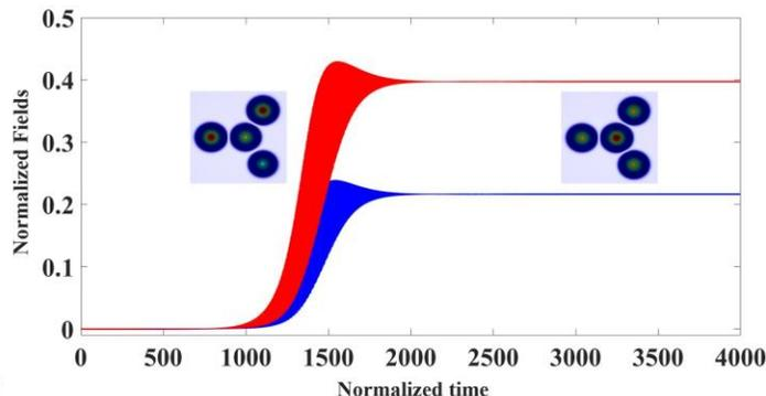
**Fig. 2.** Filed evaluation of the laser system composed of three lasers cavities coupled to the central cavity which is slightly detuned with respect to  $\omega_0$ . Here,  $k=1$  is normalized coupling,  $\frac{1}{\tau_p}=0.1$  and  $G_i=0.105$  for each cavity and central cavity has higher gain ( $1.1G_i$ ). This enhances the  $Q$  of the in-phase mode as a result decreases its threshold.
