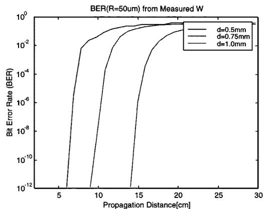
Fig. 5. BER to determine the interconnect distance.
