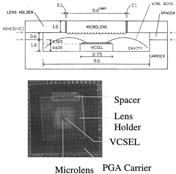
Fig. 2. (a) A detailed drawing for a transmitter packaging and (b) photo of packaged VCSEL with microlens array.
