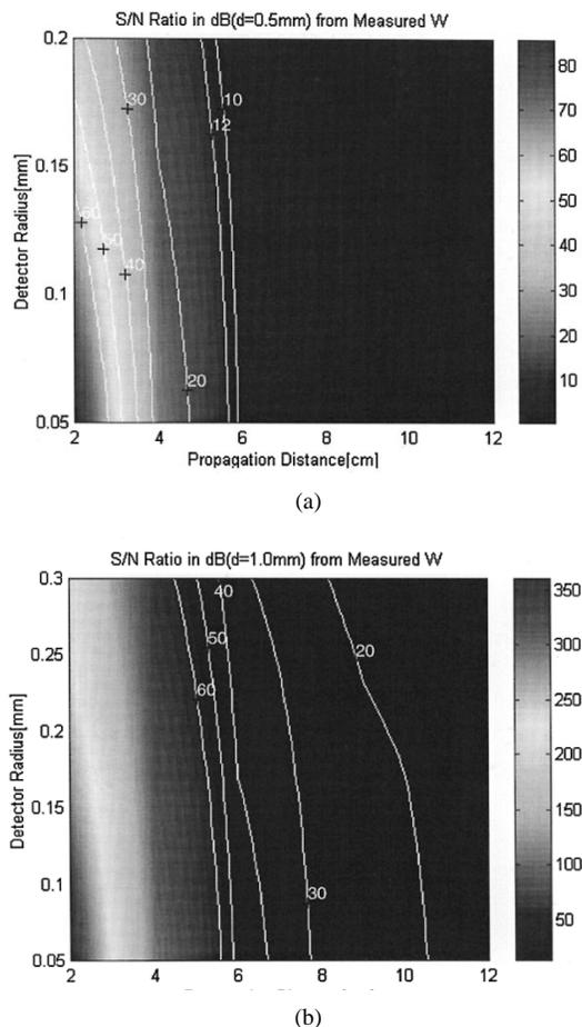
Fig. 4. SNR simulation (a) for 500  $\mu\text{m}$  array spacing and (b) for 1-mm array spacing from measured beam radius.
