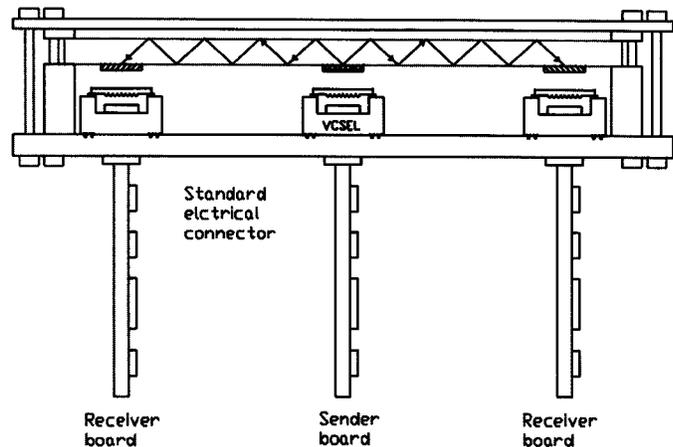
Fig. 1. Generalized optical backplane architecture for board-to-board interconnects.
