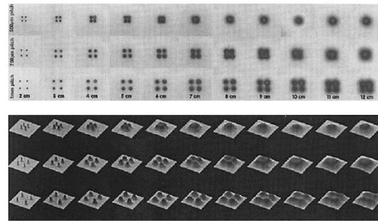
Fig. 3. Degree of overlapping between  $2 \times 2$  optical beams.
