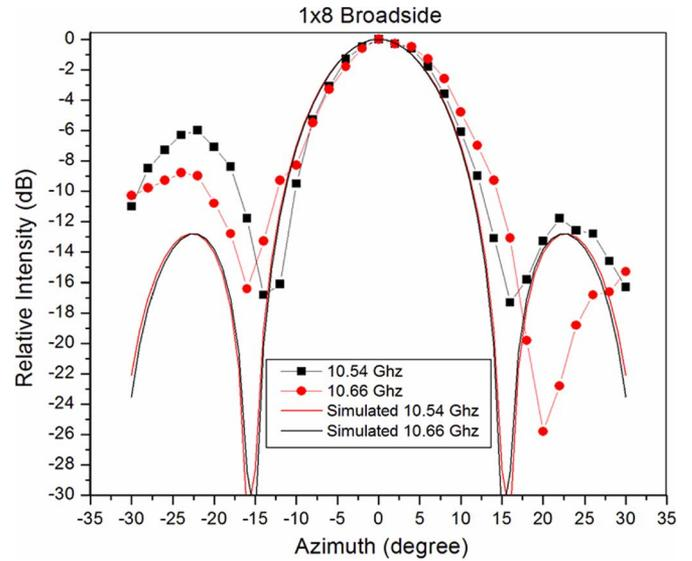
Fig. 11. Measured and simulated far-field patterns for a  $1 \times 8$  element array ( $0^\circ$  steering angle).
