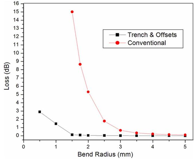
Fig. 4. Simulated bend and junction losses for the  $180^\circ$  waveguide bends ( $d = 7 \mu\text{m}$ ).
