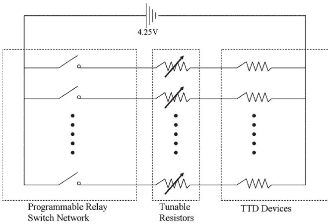
Fig. 10. Schematic of the electrical circuit used to control the optical switches.
