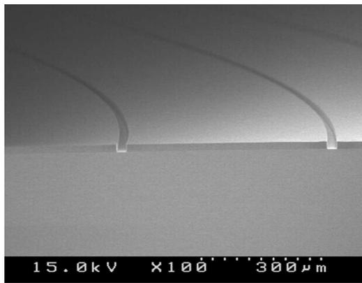
Fig. 3. SEM image of the waveguide with trench cross section.
