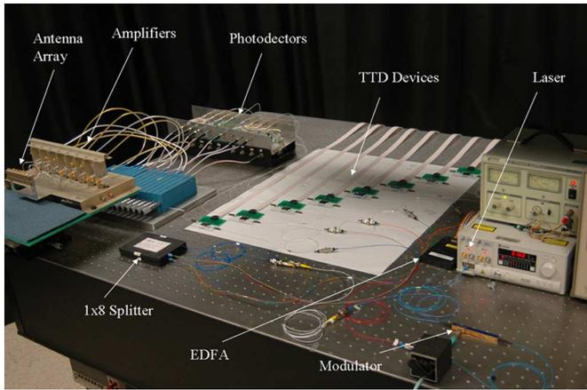
Fig. 9. Photograph of the optically delayed PAA system.
