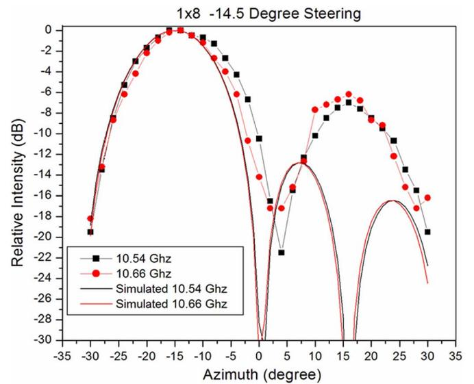
Fig. 12. Measured and simulated far-field patterns for a  $1 \times 8$  element array ( $-14.5^\circ$  steering angle).
