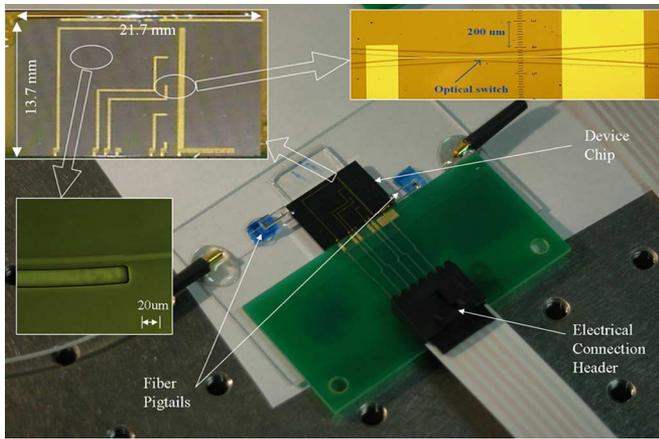
Fig. 5. Photograph of a packaged 4-bit TTD device.
