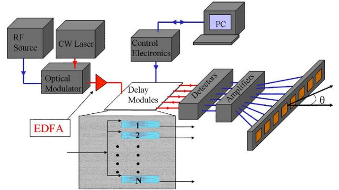
Fig. 8. Diagram of the optically controlled linear PAA system.
