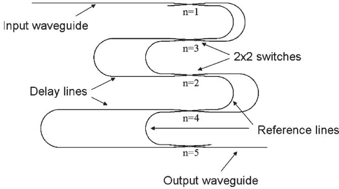
Fig. 1. TTD device structure employing waveguide optical switches and delay lines.
