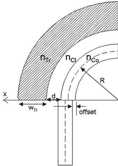
Fig. 2. Diagram of the waveguide core using offset and trench (hatched area) structures.
