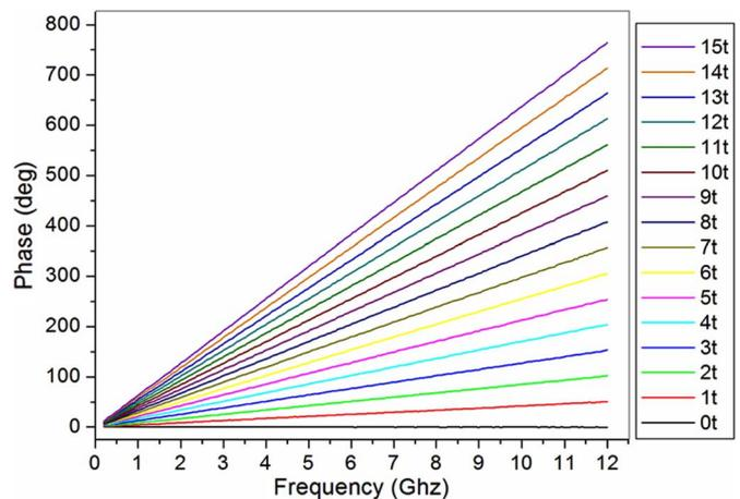
Fig. 7. Measured phase versus frequency response for each delay state.
