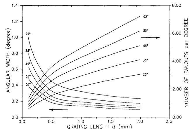
Fig. 4. Angular bandwidth and the fanout density as a function of the grating interaction length.
