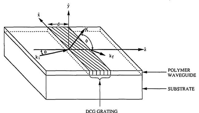
Fig. 1. Model of the polymer microstructure waveguide, with selectively defined DCG phase gratings having slanted fringes.
