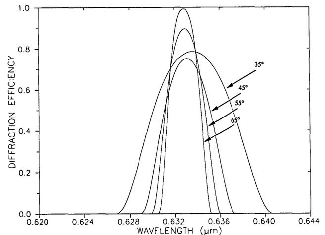
Fig. 3. Diffraction efficiency and wavelength dependence as a function of the diffraction angle  $\psi$ . A mode effective index  $N_{\text{eff}} = 1.5172$ , a center wavelength of  $\lambda = 0.6328$   $\mu\text{m}$ , an index modulation  $\Delta n = 0.01$ , and a grating interaction length  $d = 0.5$  mm were used in the calculations.
