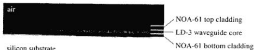
FIG. 2. Microscope photograph of the polished end face of an LD-3/NOA-61 planar waveguide. Not visible are the gold top and bottom electrodes.
