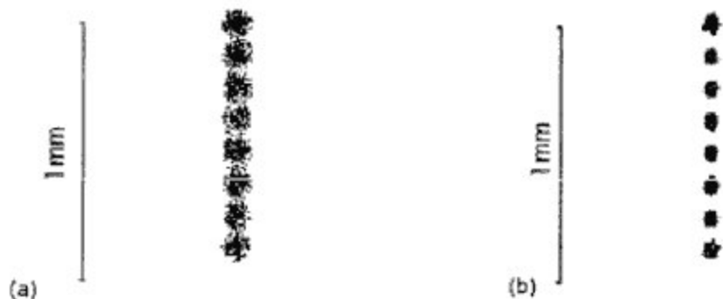
Figure 3. (a) Spot diagram of a 50 \mu\text{m} input fiber by best homogeneous lens solution. (b) Spot diagram of a 50 \mu\text{m} input fiber by axial graded index lens solution.
