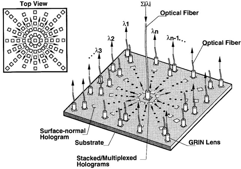
Fig. 2. Schematic diagram of a two-dimensional WDDM distributing network using substrate-guided wave optical interconnects.
