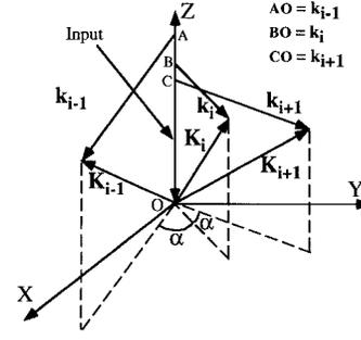
Fig. 6. Phase matching diagrams for stacked input volume holographic grating couplers.
