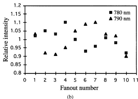
Fig. 8. Experimental results of the 2-D WDDM device while operating at 790 and 780 nm. (a) CCD image. Oblique fan-outs are for 790 nm channel. Vertical light spots corresponds to the 780 nm channel fan-outs. (b) Relative fan-out energy distributions.
