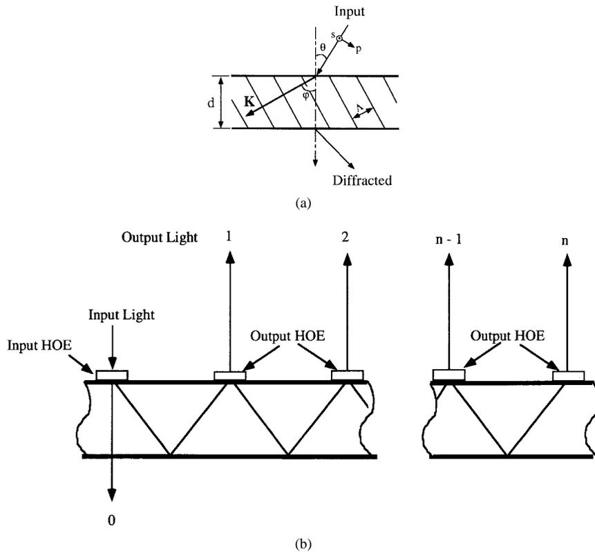
Fig. 3. (a) Schematic diagram of a transmission volume hologram and (b) a typical structure of substrate-guided wave optical interconnects.
