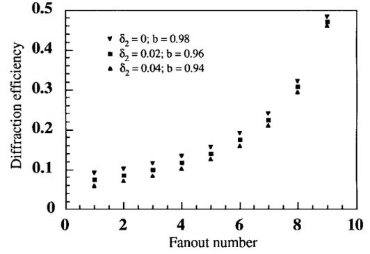
Fig. 5. Calculated diffraction efficiencies required for a 1-to-10 energy-equalized fan-out device. The last HOE, which is not shown in the figure, is with diffraction efficiency of 93% for the three cases.
