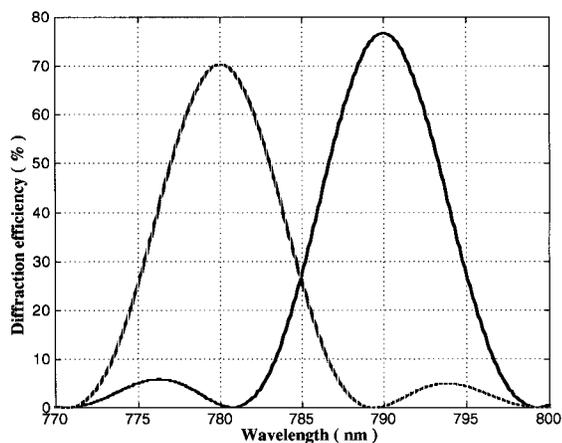
Fig. 7. Simulation results of diffraction efficiencies versus the wavelength deviation from central wavelengths 780 and 790 nm of a randomly polarized wave for 100- $\mu\text{m}$  thick photopolymer films.
