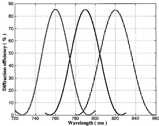
Fig. 9. Simulation results of diffraction efficiencies versus the wavelength deviation from central wavelengths 760, 790, and 820 nm of a randomly polarized wave for 20- $\mu$ m thick photopolymer films.
