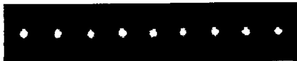
Figure 4 Far field image for a 1-to-9 optical fan-out device.
