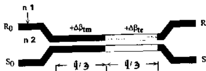
Fig.6. A directional coupler with two perpendicularly poled sections.
