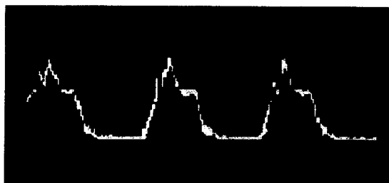
Figure 5. Receiver output from the transceiver system incorporating the bidirectional optical backplane bus for a 1.2 Gbit/sec input signal.
