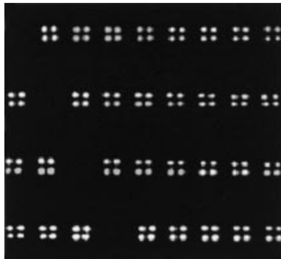
Fig. 1. (a) Generalized bidirectional optical backplane architecture and (b) experimental demonstration using 2-D array with first, second, third, and fourth channel functioning as the input coupler.
