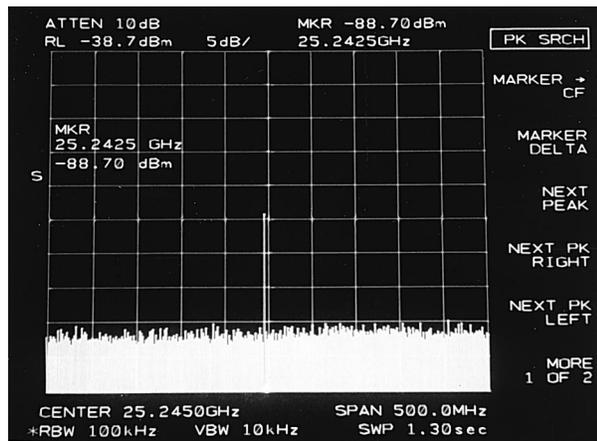
Fig. 5. 25-GHz optical heterodyne signal detected by a spectrum analyzer.
