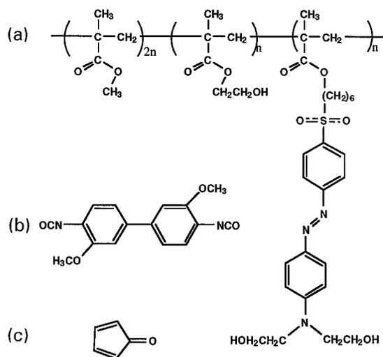
Fig. 1. Chemical structures of the LD-3 polymer solution system: (a) the LD-3 polymer, (b) the cross-linker, (c) the solvent.
