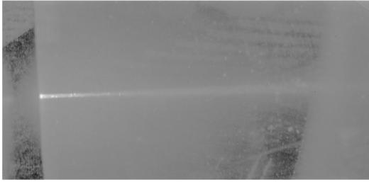
Fig. 2. Photograph showing the fundamental-mode propagation inside the LD-3 polymer waveguide that has a thickness of  $1.2 \mu\text{m}$  at  $\lambda = 632.8 \text{ nm}$ ; the waveguide length is  $4 \text{ cm}$ .
