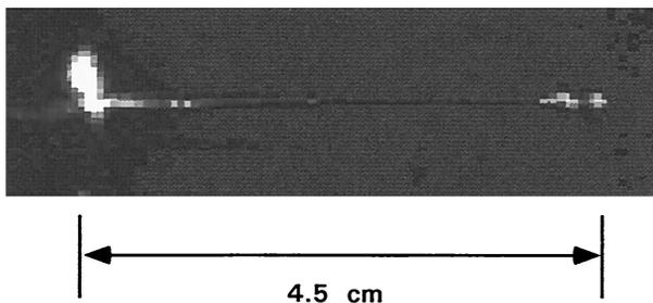
Fig. 3. CCD image of  $1.32\text{-}\mu\text{m}$  light propagation on a waveguide made on a silicon substrate. Cladding material NOA61, lower cladding  $3 \mu\text{m}$ , upper cladding  $1 \mu\text{m}$ .
