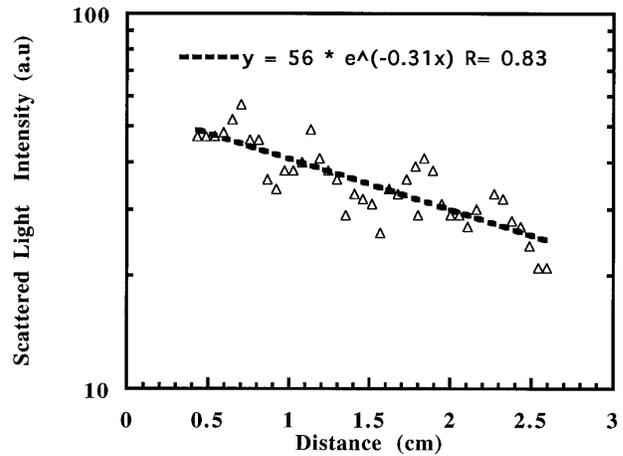
Fig. 4. Measured waveguide loss of LD-3 thin film ( $1.2 \mu\text{m}$  thick) on a silicon substrate at  $\lambda = 1.32 \mu\text{m}$ .
