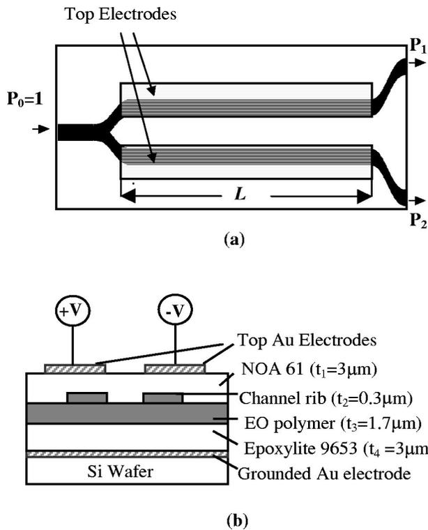
FIG. 1. Schematic diagram and fabrication parameters of the  $1 \times 2$  Y-fed coupler modulator. (a) Top view. (b) Cross section. The channel width was  $4 \mu\text{m}$ . The separation between the two channels was  $6 \mu\text{m}$ .
