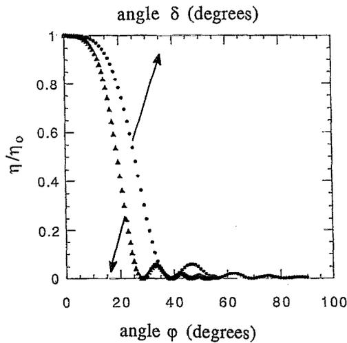
FIG. 5. Normalized coupling efficiency ( $\eta/\eta_0$ ) of the near-surface-normal fanout beams as functions of angles  $\delta$  and  $\phi$ .
