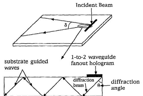
FIG. 1. Schematic of the demonstrated 1-to-2 intraplane interconnects with a surface-normal incident beam.
