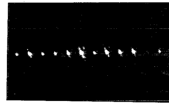
FIG. 4. (a) Reconstruction of the surface normal optical interconnect. Surface normal interconnection is not clear in this photograph due to the overlap between the diffracted beams and the undiffracted beam. (b) Near-field pattern of the 12 surface normal beams coupled out of the total internal reflection hologram array shown in Fig. 1. The separation between the two nearest beams is 2 mm.
