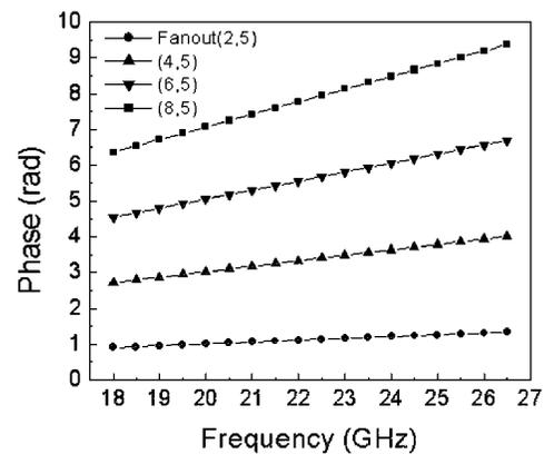
Fig. 2. Measured phase as a function of frequency of the fifth column fan-outs. The delayed signal is measured with respect to the (1,5) fan-out. The time delays of (2,5), (4,5), (6,5), (8,5) are calculated to be 8.04, 24.12, 40.20, and 56.28 ps from the slope of the phase versus RF frequency.
