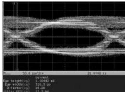
Fig. 5. Eye diagram of a 2.5-Gb/s random digital signal after the optical TTD link measured by HP 83480A Digital Communications Analyzer.
