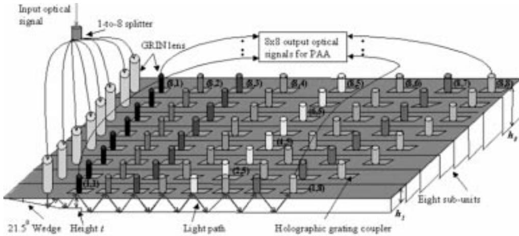
Fig. 1. Schematic of the TTD module. The TTD module is composed of eight subunits with holographic-grating couplers on top of the substrates. The input signals are coupled vertically into the module using graded index (GRIN) lenses. A portion of the substrate guided wave is extracted out each time the wave encounters the output holographic-grating coupler and focused back into optical fibers using GRIN lenses.
