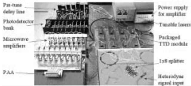
Fig. 3. Picture of the integrated K-band PAA system.
