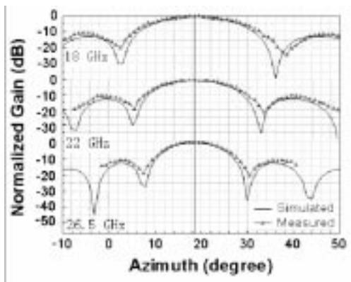
Fig. 4. Comparison of far-field patterns of the PAA at  $18.5^\circ$  scanning angle at three different frequencies: 18, 22, and 26.5 GHz. Solid curves show simulated results and curves with triangles show the measured data.
