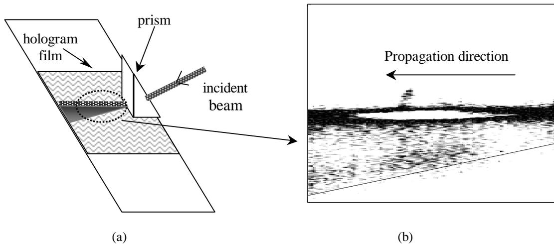
**Figure 1** (a) Experimental configuration. A hologram film is carried on a microscopic slice. A high index prism is used to couple light into the film. (b) Magnified part of the film (a real photo): A narrow beam light propagates in holographic grating from right to left almost horizontally, spreading over a triangular region. The lower border of the triangle is indicated by a thin drawn line as predicted by theory.
