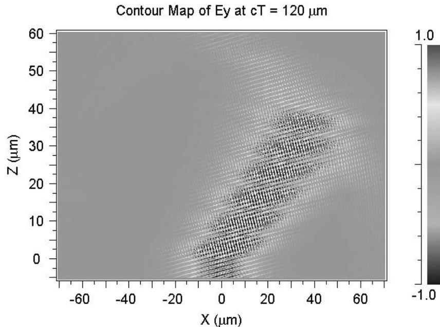
**Figure 3** A well defined beam in the case of “negative refraction.” (triangular lattice  $a=1$  mm,  $n_0=1.5$ , sinusoidal index modulation amplitude 0.3,  $w_0=30$  mm,  $AOI=-9.5^\circ$ , beam deflected by  $54.5^\circ$ )
