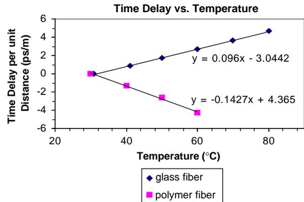
Fig. 4. Time delay per unit length of fiber plotted against temperature for silica and polymer fibers. The silica fiber was 45 m long and the polymer fiber was 7.66 m. The plots are linear showing the time delay is directly proportional to the temperature of the fiber.
