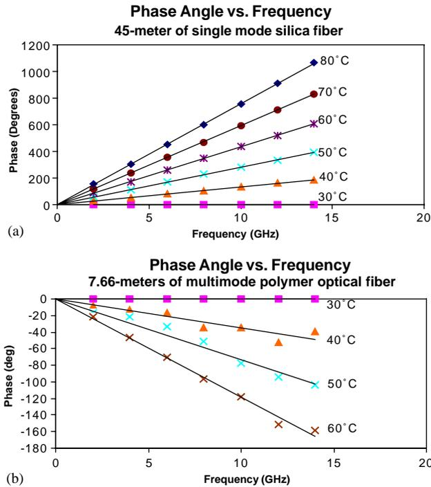
Fig. 3. Measurement results showing the phase angle as a function of frequency for (a) 45-m section of Corning LEAF silica fiber, (b) 7.66-m section of Lucina polymer optical fiber. Larger slopes, as the temperature increases, represent greater amounts of time delay.
