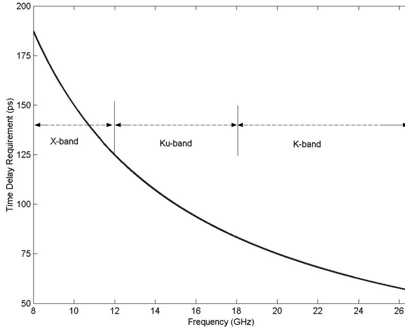
Fig. 1. Time delay needed as a function of RF frequency for a 4x4 element sub-array.
