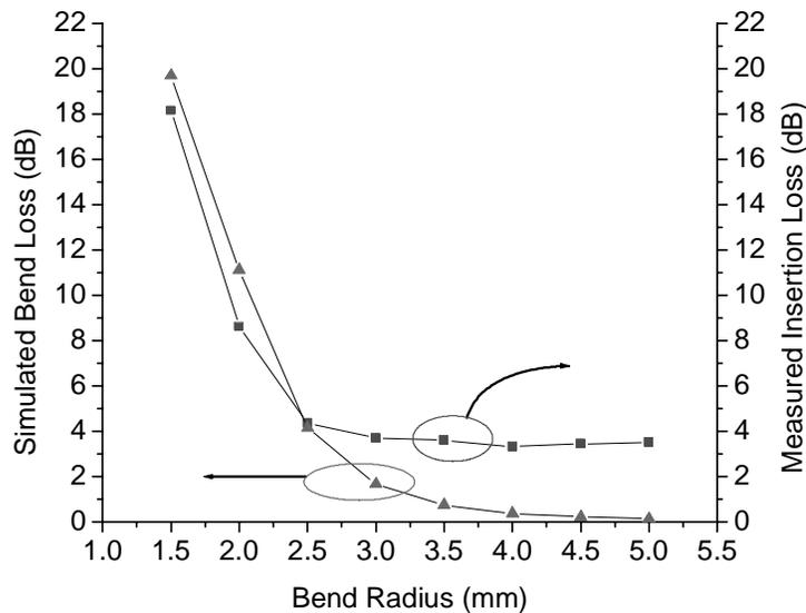
Fig. 6. Simulated bend losses and measured insertion losses for 180 degree bend.
