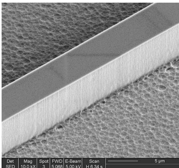
Fig. 4. SEM image of a channel waveguide core etched with the optimized RIE parameters.
