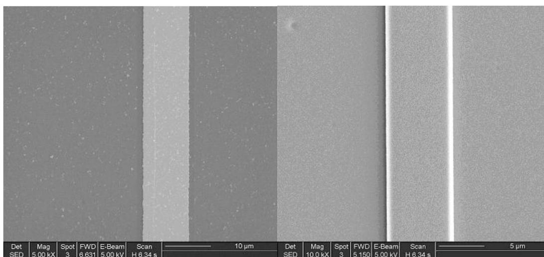
Fig. 5a.(left) Patterned hard mask of Cr/Au material and 5b(right) Patterned SiO<sub>2</sub> hard mask.
