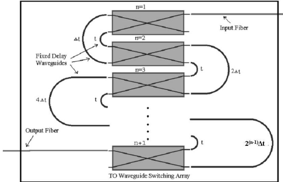
Fig. 2. TTD device structure employing waveguide optical switches and delay lines.
