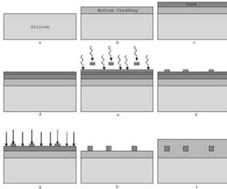
Fig. 3. The polymer waveguide fabrication process.
