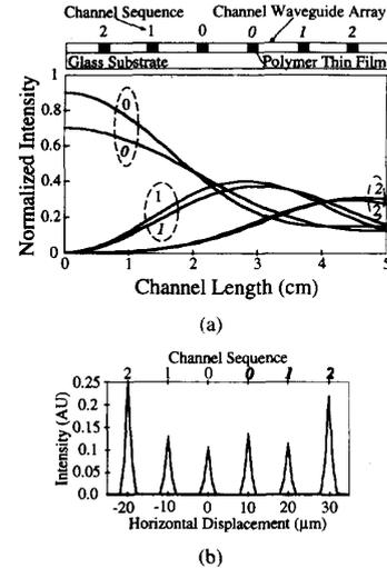
Fig. 5. (a) The intensity distribution in a PBSMBA based on (7) using the experimental parameters of Fig. 4, where  $n = \infty$  was assumed. (b) The transverse intensity distribution at  $z = 5$  cm.
