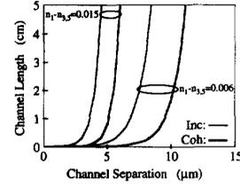
Fig. 2. Channel length versus channel separation to ensure a minimum of 32 dB and 12 dB S/N ratio for coherent light sources and incoherent light sources, respectively.  $n_1 = 1.5$ ,  $n_2 = 1.0$ , and  $\lambda = 0.6328 \mu\text{m}$  were assumed.
