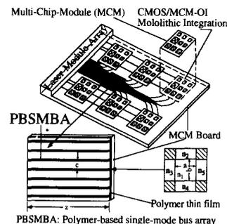
Fig. 1. A schematic diagram of a MCM board using PBSMBA, where the cross-section of a channel waveguide under consideration is also shown.
