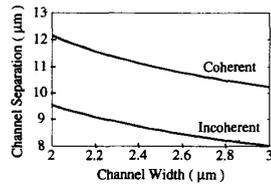
Fig. 3. Channel separation versus channel dimension based on (6) and (7).  $z = 5$  cm,  $a = b = 2$   $\mu\text{m}$ ,  $n_1 = 1.5$ ,  $n_2 = 1.0$ ,  $n_1 - n_4 = 0.01$ , and  $n_1 - n_{3,5} = 0.006$  at  $\lambda = 0.6328$   $\mu\text{m}$  were assumed.
