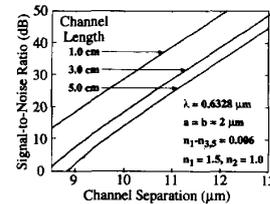
Fig. 6. Signal-to-noise ratio versus channel separation as the parameters of channel length.
