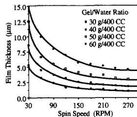
Fig. 7. Film thickness as a function of the spin speed with different gel/water ratios as a parameter.
